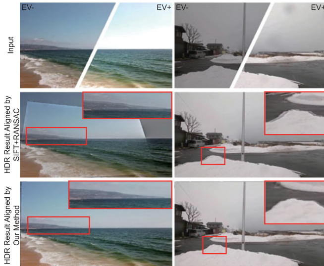
Fig. 10. Results of HDR imaging from Exposure Fusion. Different exposures should be well aligned before the HDR fusion. The second row shows the fusion results of SIFT+RANSAC while the third row shows the results aligned by our Deep Homography.
