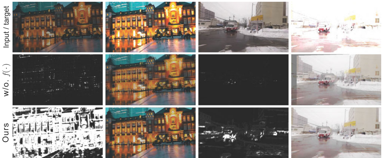
Fig. 3. Ablation study on the effectiveness of our feature extractor, demonstrated by examples with illumination change, displayed separately in the left and right two columns. For each example, the input and target GT images are in Row 1, followed by the results by disabling the feature extractor f(\cdot) (Row 2) and by ours (Row 3), including the learned masks and the aligned results in odd and even columns. As seen, our results are obviously stable for such a case.
