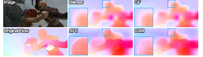
Fig. 8. An example of using our AFU module to upsample optical flow in the pyramid network. We first downsample the ground-truth optical flow (original flow) by 64 times, which is the smallest scale of our pyramid network. Then we upsample the downsampled flow to the original size using our AFU, bilinear method, guided filter [53] (GF) and the learned convex upsample module [12] (CUM). Compared with previous methods, our AFU can preserve more object structure in the upsampling process.
