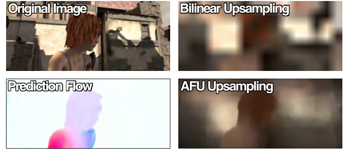
Fig. 9. An example of using our AFU module to upsample images. We first downsample the original image by 64 times, which is the smallest scale of our pyramid network. Then we iteratively upsample the downsampled image to the original size using our AFU, as Eq. 11. Compared with bilinear upsampling, our AFU upsampling can preserve detail object structures.
