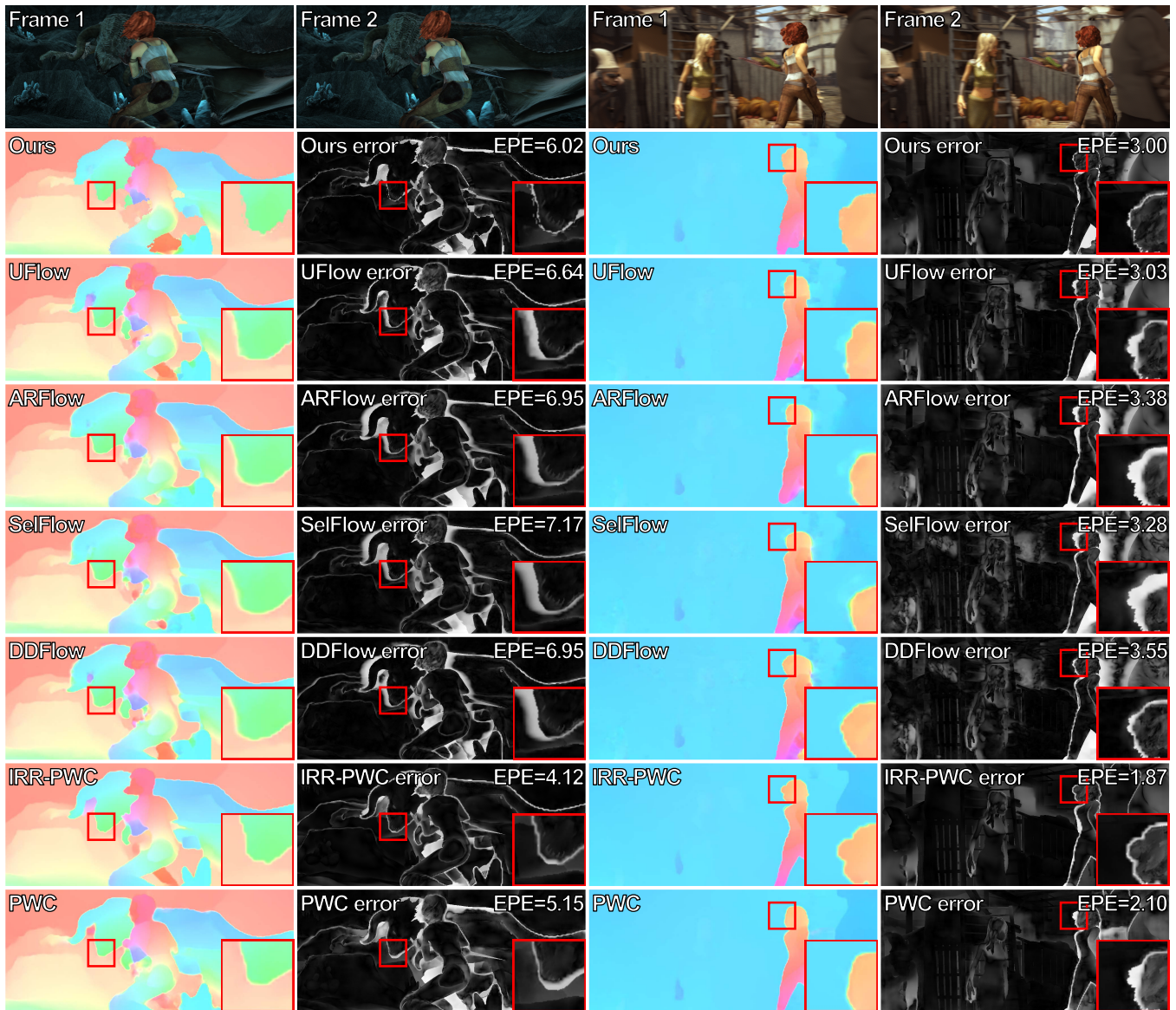
Fig. 8. Comparison on MPI-Sintel Final benchmark, where results of other unsupervised methods UFlow [59], ARFlow [58], SelFlow [32] and DDFlow [31] are shown. Results of fully supervised methods PWC-Net [40] and IRR-PWC [35] are shown in the last two rows. The error maps of the predictions are visualized in the even columns. For better visualization, the zoom-in views of some local patches are depicted in the right bottom corner of each sample.
