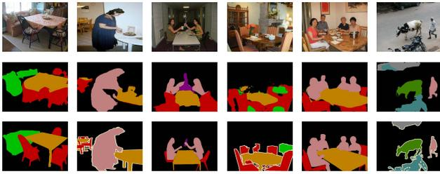
Fig. 11. The segmentation results of multiple classes on the PASCAL VOC 2012 dataset by our method. The first row, second row and third row show the original images, the segmentation results and the groundtruths, respectively.
